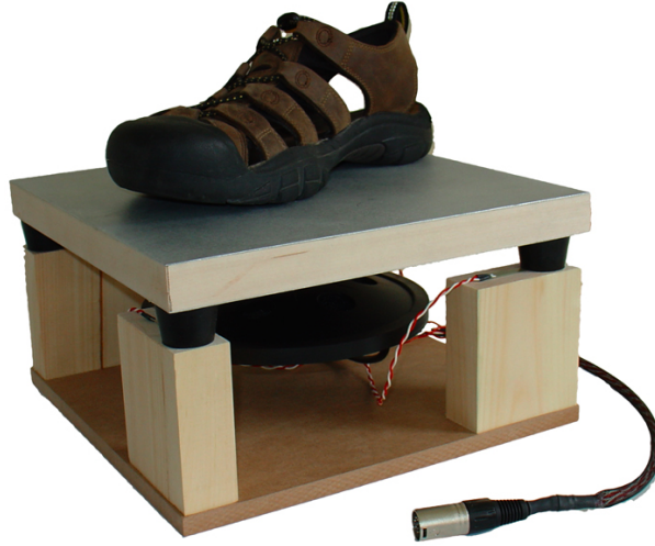
Fig. 2.2: Photo with large mens' shoe, showing representative size. The model shown is based on the low-cost force sensing resistor option. The cable in the foreground interfaces the sensors with the data acquisition unit.
