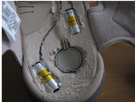
Fig. 2.5: Photograph of pressure sensor and of two actuators embedded in the shoes.
