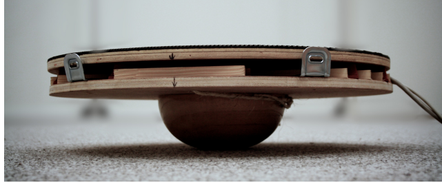
Fig. 2.9: Actuated and instrumented wobble board.
