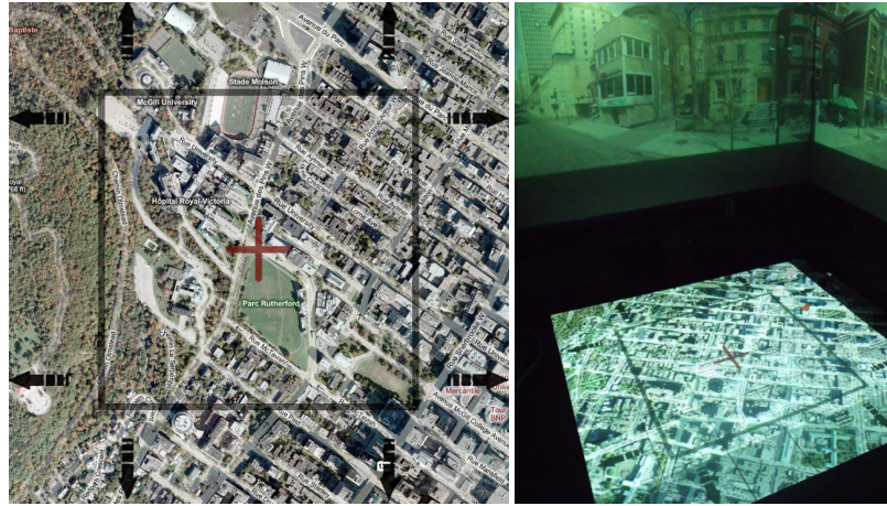
Fig. 3.13: The “magic tape” interface: A rectangular outline indicates the magic tape boundary, beyond which, the user’s footstep will result in panning in the direction formed by a vector from the center crosshair and the user’s foot.
