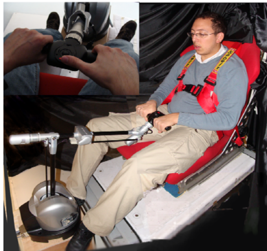
Figure 12. Experimental apparatus used for generating “Haptic Motion”: A force-feedback is sent in the hands of the user in a synchronized way with visual feedback of motion in the VE.
