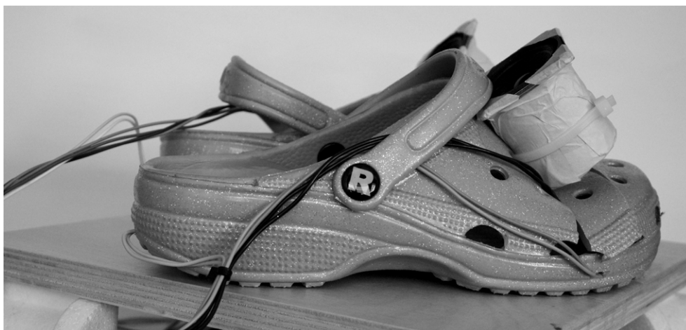
Figure 7.1: First shoe mock-up made with rubber clogs: speakers setting.
