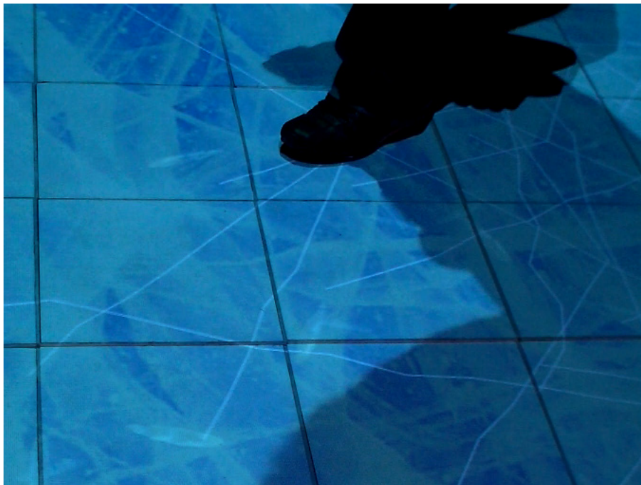
Figure 8.1: Still image from video documentation of an illustrative interactive scenario in which the multimodal synthesis and contact sensing techniques described in this deliverable, and in D3.1, are used to allow users to walk over a virtual pond whose surface has frozen over. Cracks in the virtual ice sheet dynamically form at loci of contact between feet and floor.
