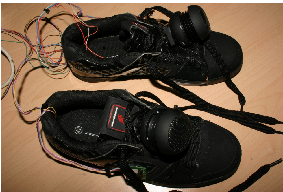
Figure 7.2: Second shoe mock-up made using sneakers: speakers setting.
