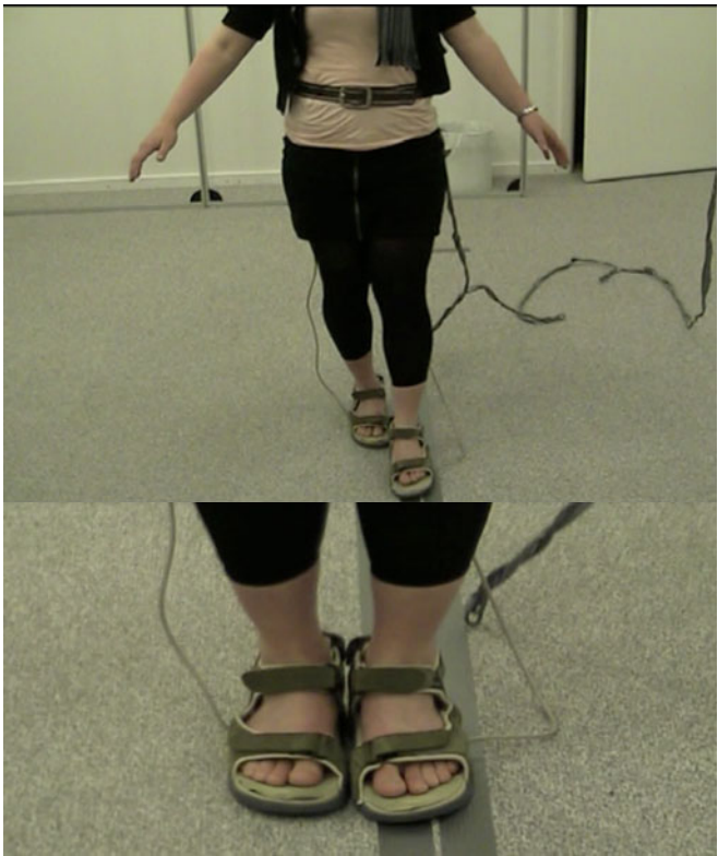
Fig. 3. Top: A user wearing the sandals enhanced with sensors and actuators. Bottom: the sandals.
