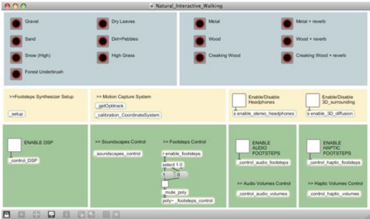
Figure 3.4: A screenshot of the audio-haptic synthesis engine used in the architecture.
