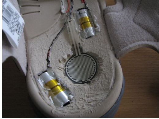
Figure 3.3: A picture of one pressure sensor and two actuators embedded in the shoes.
