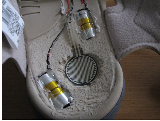
Figure 2.7: A picture of one pressure sensor and two actuators embedded in the shoes.
