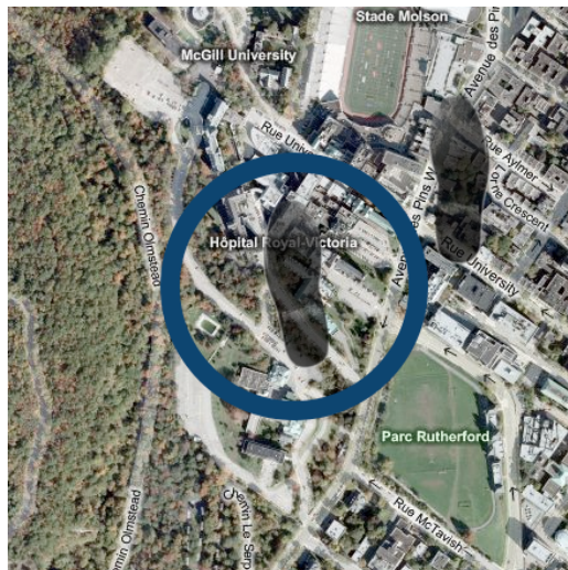
Figure 2.3: Here, the first foot establishes the pivot point, and the second foot slides or drags the display in a scrolling motion, with inertia.
