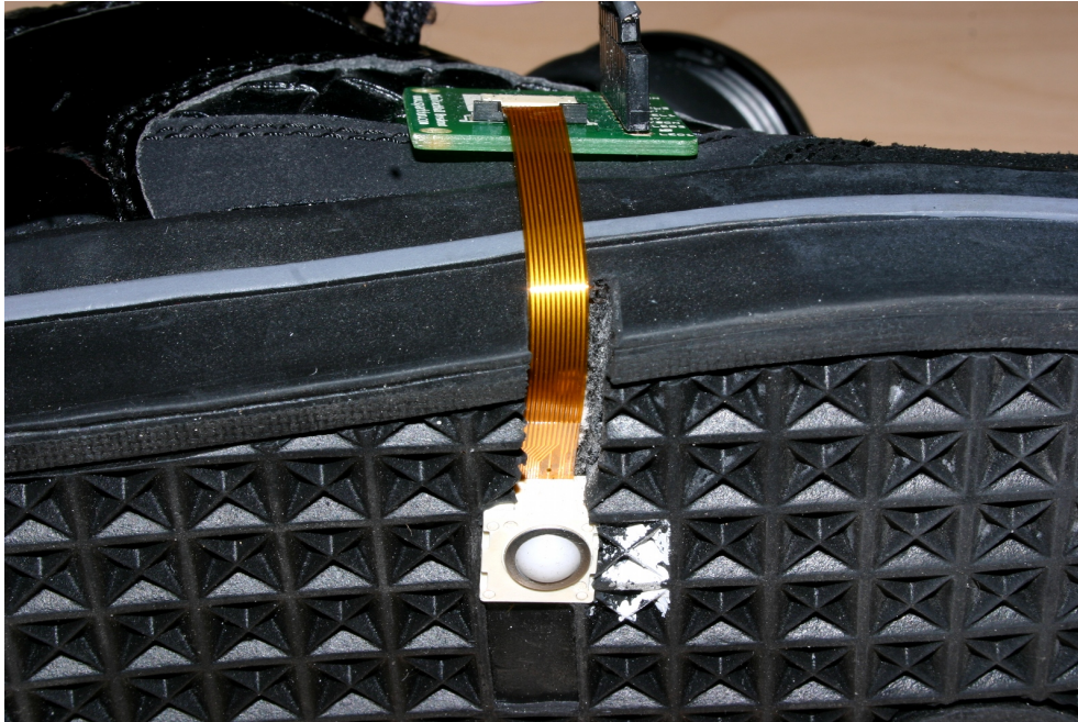
Figure 3.8: Second prototype: the trackball.
