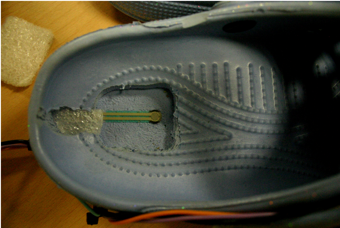
Figure 3.5: Physical placement of sensors in the first prototype. Some pieces of rubber are placed on the sensors in order to protect them and to transmit force from the bottom of the foot to the active layer of each of them.
