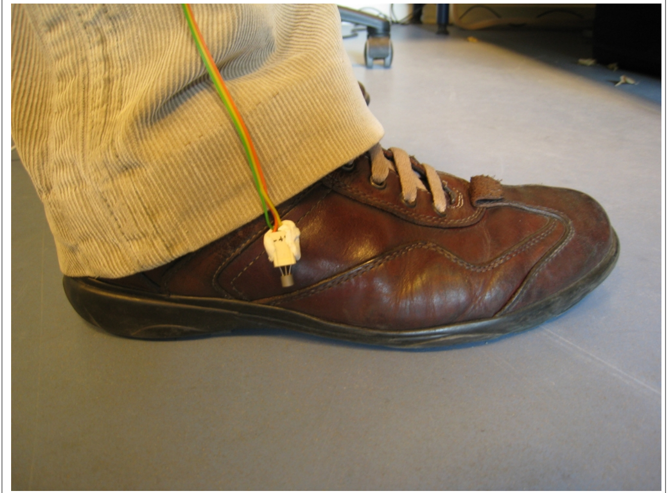
Figure 4.1: The contact microphone attached to the shoe.
