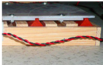
Figure 2.5: Compact structural elastomeric elements able to resist large vertical loads and yet remain compliant lateral independently from the load.
