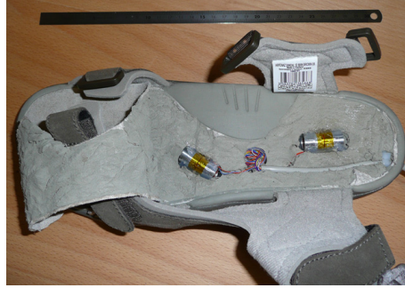
Figure 2.7: Active shoe (exploded to expose the actuators) made of commercial components.
