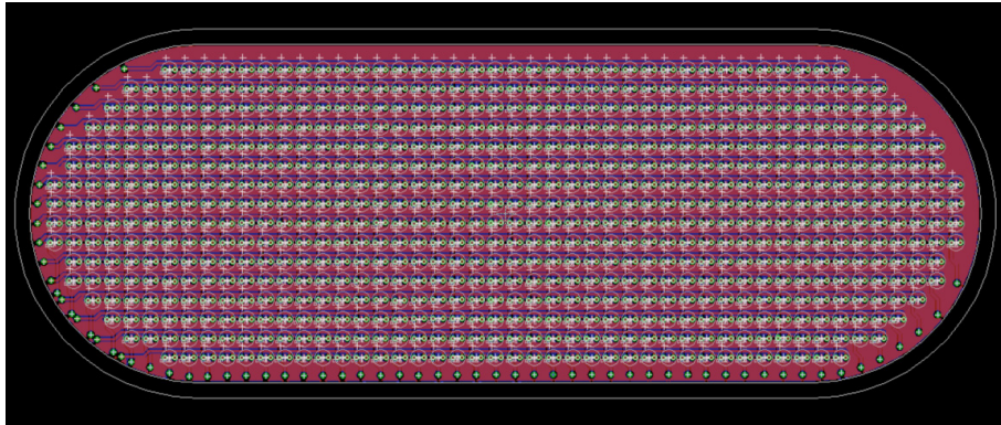
Figure 2.9: Signal routing upper board of the Spatial Tactile Display Layer.
